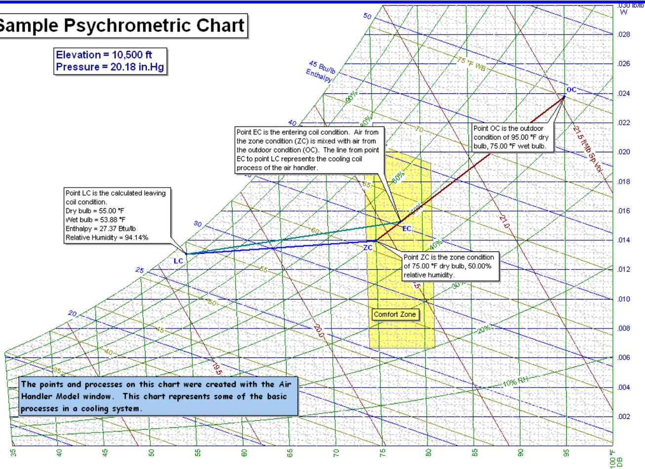
Point LC is the calculated leaving coil condition.
